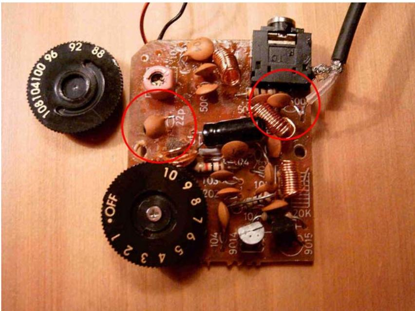
Figure: One 22 pF capacitor lifted on the right-hand side near the headphone connector for connection to the external antenna, and another one lifted on the left-hand side, above the volume control for increasing the tuning range (The receiver IC is on the foil side of the board).
