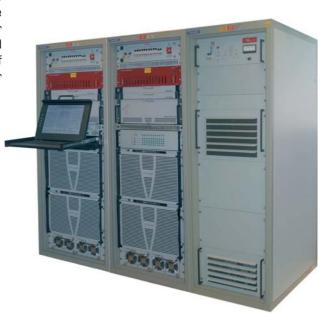
The HF SDR as a complete transceiver can operate independently or within a totally integrated end-to-end naval communications system offering voice, data, messaging and e-mail services. Based on open systems architecture principles the design provides a fully supported software environment enabling ready adaptation or enhancement as operational needs change. It can evolve to meet the changing needs of the naval communications community and the demands of future warship design.
