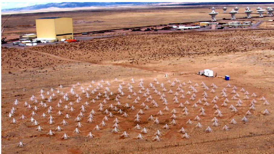
Figure 1: Aerial view of LWA1, the first station of the Long Wavelength Array (LWA), located near the center of the National Radio Astronomy Observatory's Jansky Very Large Array (VLA) telescope in New Mexico. LWA1 operates over 10-88 MHz and consists of 256 cross-dipole antenna stands arranged in a semi-random pattern. The diameter of the station is approximately 100 meters. Parabolic VLA antennas appear in the background at top right. The LWA1 is led by the University of New Mexico and supported by the National Science Foundation as a University Radio Observatory.
