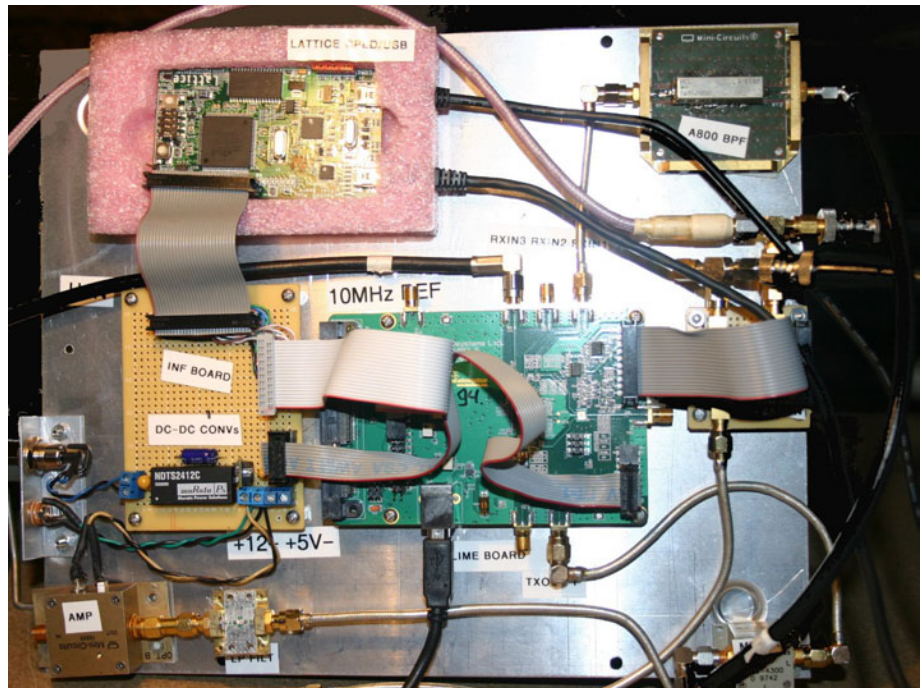
Figure 1 – the benchtop RASDR. The Lime board (green) is in the center, while the Lattice digital board is shown at the upper left.
