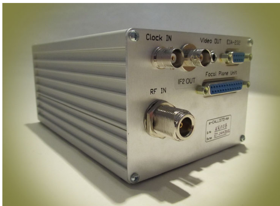
Figure 4 – Panel modifications of a CALLISTO Receiver showing the BNC connector added to the rear panel to the right of the Clock Input connector. This connector also can be used with both the wideband and narrowband modifications.
