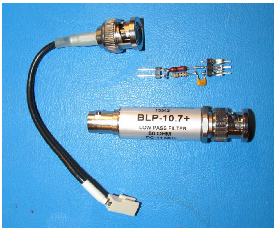
Figure 3 – Components required for the wideband down-converter modifications. In my experimental radio, I used pluggable interfaces and a commercial lowpass filter because it was available in my lab. A home-made filter may be used but the IF output response may differ from that shown later in this article. The cost of the parts shown here is about US$40.
