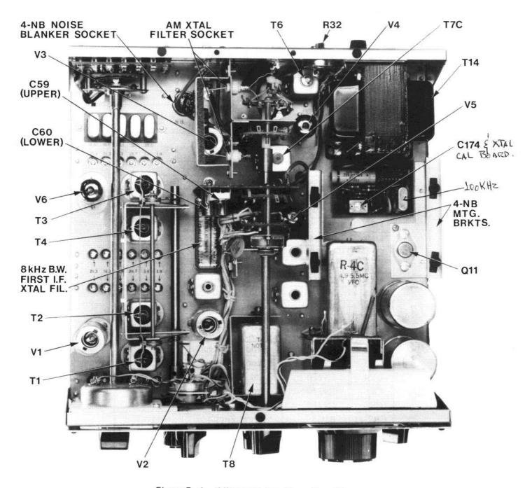
Figure 5-1. Alignment Locations, Top View
