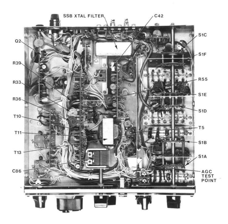
Figure 5-2. Alignment Locations, Bottom View
