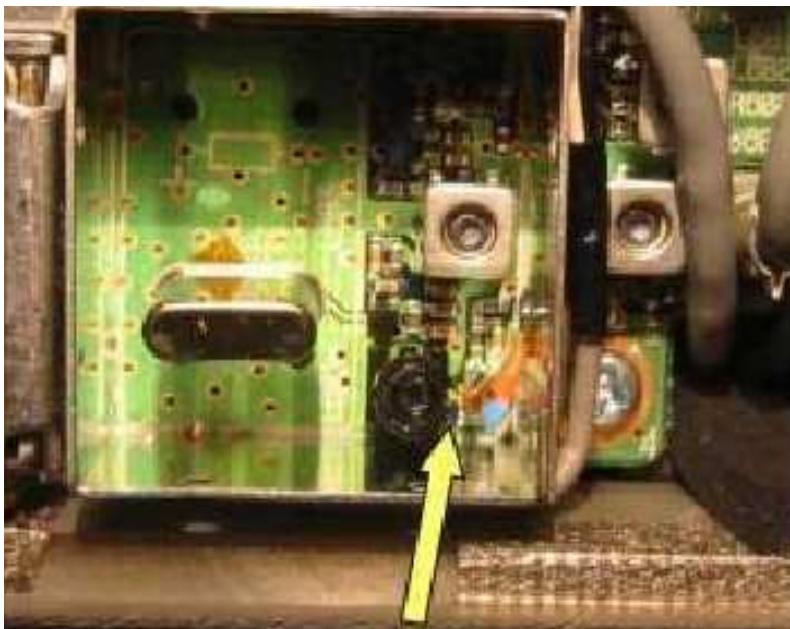
Picture 3: diode is right next to the L601
