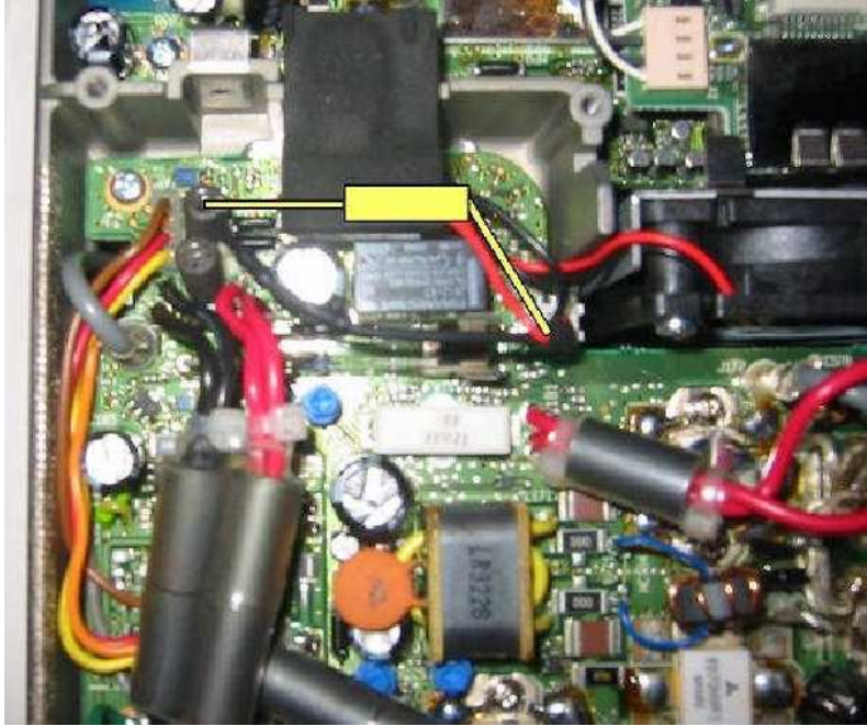
Picture 4: Position of resistor
