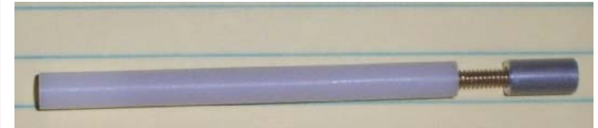
PTO coil form w/ tuning rod
